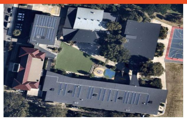
Rainbow Street Public School has installed one of the largest solar power systems on a primary school in the Eastern Suburbs. The systems 326 panel's will produce clean, green energy to power the schools facilities for many years to come. The system was funded and installed as part of the 2017-18 rebuild of the school and forms an integral part of School Infrastructure NSW (SINSW) sustainability programs.
